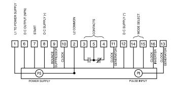
TERMINAL WIRING SOLID STATE OUTPUT MODULE
