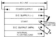
**B. DC VOLTAGE** (sustained *start* signal) The *start* voltage must be on throughout the count cycle. The 354 is ready to count whenever the voltage reaches +4.5 or -3V DC; it resets when the voltage drops to +1 or -1V DC.
