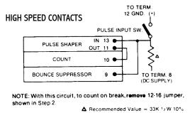
C. DC VOLTAGE PULSES. In this circuit, the 354 counts when the voltage decreases from above +4.5V to below +1V, or from above -3V to below -1V, with a jumper installed between Terminals 12 and 16 as shown in Section 2; to reverse the action, simply remove the jumper.
