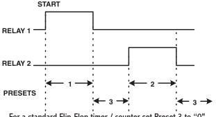
For a standard Flip-Flop timer / counter set Preset 3 to "0".
