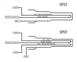
Figure 4. Schematic
