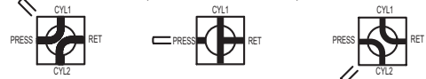
HANDLE ORIENTATION (AS SHOWN CW) (ACTUATOR PORT 'B' PRESSURIZED) HANDLE CENTERED (MANUALLY OVERRIDE ONLY) HANDLE ORIENTATION (AS SHOWN CCW) (ACTUATOR PORT 'A' PRESSURIZED)
