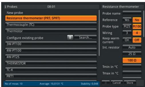
In this menu the probe settings can be selected and the reference thermometers can be stored under a unique name.
