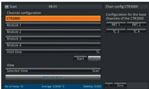
In this menu the user can define a scan by selecting the channels and the hold time. For activating the scan use the start button.
