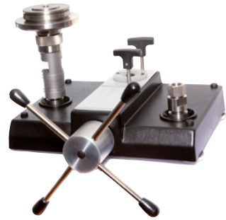
Model CPB3800 pressure balance
