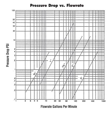
For estimating pressure drops on liquids other than water, use the following formulas:
