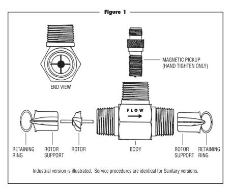
The turbine flowmeter should be installed in a location where the process line will remain full of liquid at all times. Otherwise, when the process line becomes empty and a valve is opened, the high velocity fluid hitting the turbine flowmeter rotor can cause severe damage.
