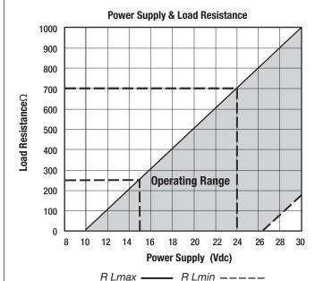
$\mbox{ Maximum load resistance } \begin{tabular}{ll} $R_{Lmax}$ & $\frac{E\left(V\right)$-$10(V)}{0.02(A)}\left(\Omega\right)$ \\ \end{tabular}$
