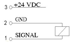
The reference point for the PNP-output is GND (GROUND = 0 VDC).
