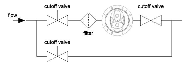
For proper operation the flowmeter must be purged of air. During long periods of inactivity or after a flushing, air may be in the piping. Elimination of the air may be achieved by operating the meter at a low flow rate until all the air is eliminated. Damage may occur to the flowmeter if it is run above the maximum rated flow rate or if the maximum differential pressure of 15 psi (1 bar, 100 kPa) is exceeded.
