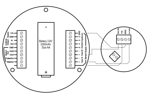
7.4.4 For Z2/Z8/Z9 electronics options (2 Hall sensors for direction detection)
