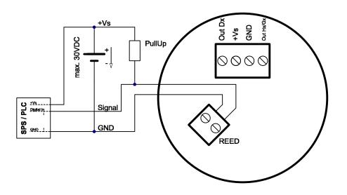
The individually specified maximum electrical values of the reed switch must never be exceeded, even for a moment. Higher switching values may reduce the service life or even destroy the contact.
