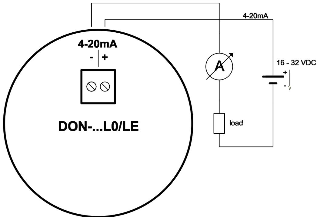
All DON devices with L0/LE options are factory-calibrated to the respective measurement range end value. This setting should only be modified by the manufacturer.
