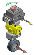
The image to the left shows a TopWorx<sup>™</sup> unit mounted parallel to the process valve in the closed position. The green arrow at the top shows the "normal acting" direction of travel to open the valve. This is the standard orientation and unless otherwise specified, your unit will be factory set to operate in this fashion.
