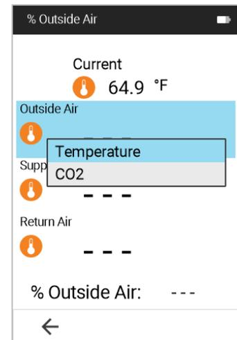
The **Percent Outside Air** feature offers the choice between using Temperature or CO<sub>2</sub> for the Percent Outside Air study if a probe that supports either CO<sub>2</sub> or Temperature is plugged in.
