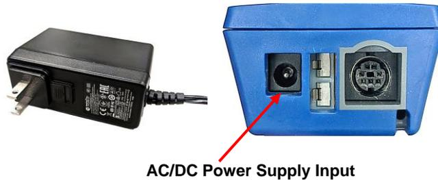
When the AC/DC power supply is connected, the instrument will automatically turn **ON**. To turn the instrument off, disconnect the AC/DC power supply. If batteries are installed, press the power button for 3 seconds.
