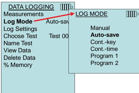
When set to **Auto-save**, the Sample Time can be adjusted. Sample Time is the time period over which the Sample will be averaged.
