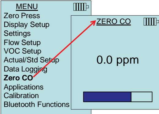
**NOTE:** The Zero CO function should be performed in an area where no combustion is taking place which may affect zeroing of the sensor.
