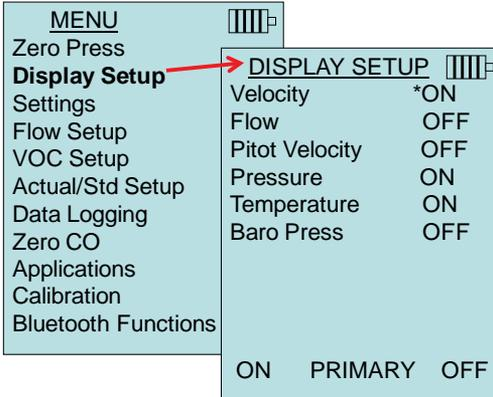
**NOTE:** Pitot Velocity and AFProbe Velocity cannot both be ON at the same time, nor can one be set to **PRIMARY** and the other to ON. Only one can be ON at any given time.
