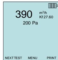
**NOTES:** The horn numbers are the models of the horns. For example, 100 refers to a horn model number AM 100. Only horns with Model numbers as follows can be used with this function: AM 100, AM 300, AM 600 and AM 1200. If a horn model number is chosen, the instrument will return to measuring mode and use a preprogrammed curve to calculate flow rate from velocity when using a thermoanemometer probe.
