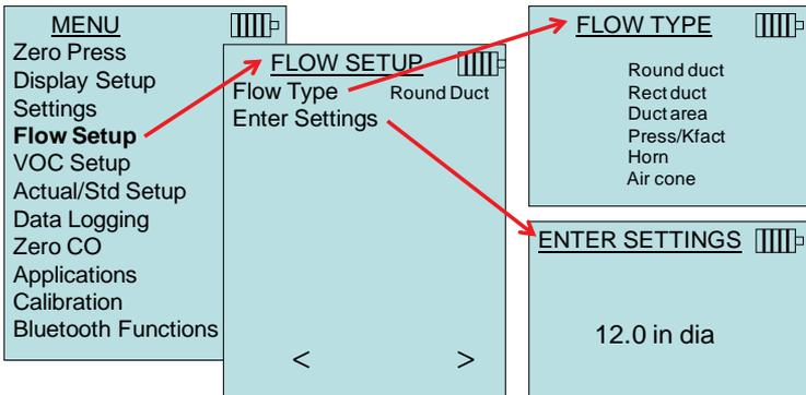
**NOTE:** Press/Kfact allows for calculating flow rate from diffusers or flow stations with pressure taps using the instruments pressure ports and Kfactors. The Kfactors are obtained from the diffuser or flow station manufacturer. For more information, refer to [Application Note TSI-114](#).
