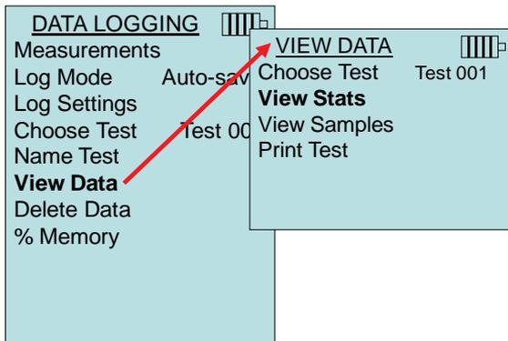
Use the ◀ and ▶ arrow keys to view statistics of all the measurement parameters stored in a Test ID.
