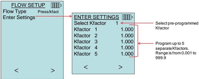
**NOTE:** When measuring flow with a Kfactor, the value can be quickly changed by pressing the ▲ or ▼ key:
