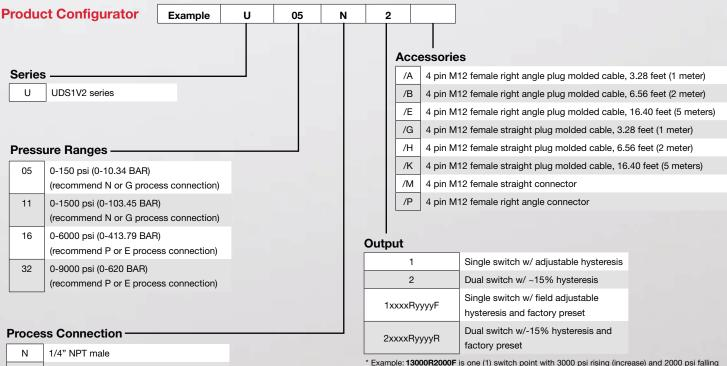
Example: 13000H2000F is one (1) switch point with 3000 psi rising (increase) and 2000 psi talling (decrease) 23000H1000R is two (2) switch points with first switch set at 3000 psi rising and second
