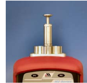
IPTR Cartridge Valve Integral valve is open and DP sensor equalized until the push button valve is depressed
