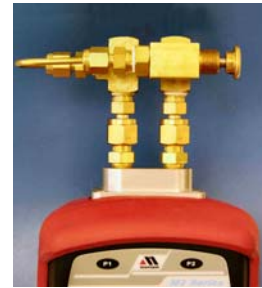
PTR Manifold Valve is open and DP sensor equalized until the push button valve is
