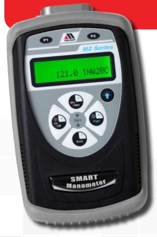
Meriam's M200LS Lab Standard Smart Manometer offers the best available pressure measurement accuracy in a portable, handheld format. The NIST traceable accuracy is typically  $\pm 0.01\%$  of F.S. and is independent of temperature effect over an operating temperature range of 59° to 86° F. Pressure ranges from 28"  $\rm H_2O$  F.S. to 500 PSIG F.S. are available.
